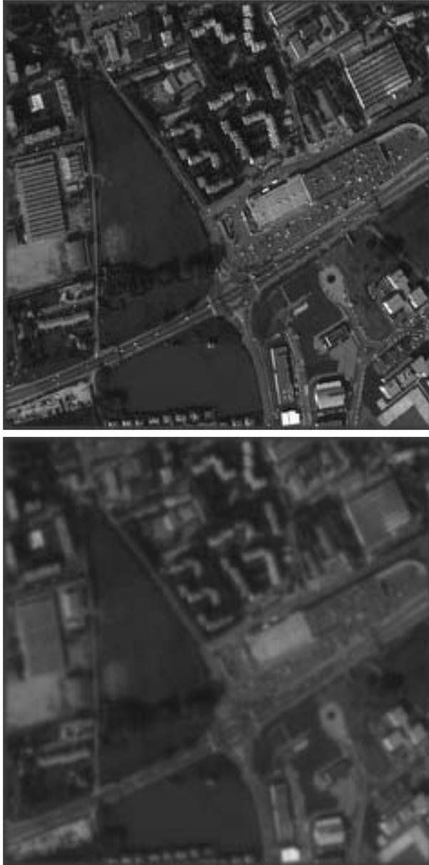
Figure 4. *Reference image and a filtered and noised image.* a) Top: reference image. b) Bottom: the data. This image has been generated applying the MTF given in (17) to the top image and adding a Gaussian white noise of zero mean and standard deviation  $\sigma = 1$ .
