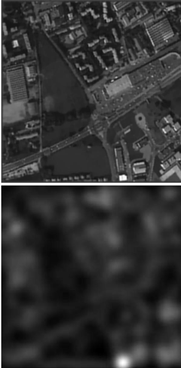
Figure 5. *Restored image with local Lagrange multipliers.* a) Top: the restored image corresponding to the data given in Figure 4.b. The restoration has been obtained using the algorithm of last section. We have used a Gaussian function  $G$  of standard deviation  $\sigma = 6$ . b) Bottom: the function  $\lambda(i, j)$  obtained.
